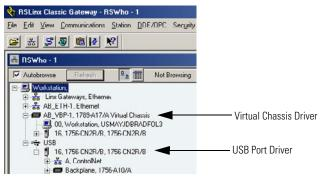
Your 1756-CN2 or 1756-CN2R module appears under two different drivers, a virtual chassis and the USB port. You can use either driver to browse through your ControlNet module.
