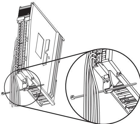
4. Wrap the cable tie around the wires and secure it.
