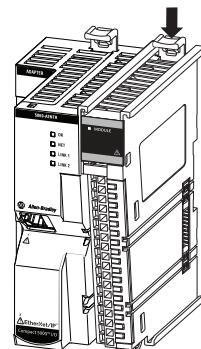
5. Pull the module away from the DIN rail.
