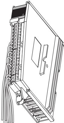
3. Thread the cable tie through the cable tie hook at the bottom of the RTB.
