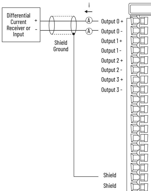
**Channel Connections** The diagram shows a device that is connected to channel 0. You are not restricted to using only this channel. You can connect devices to any channel or combination of channels as needed.
