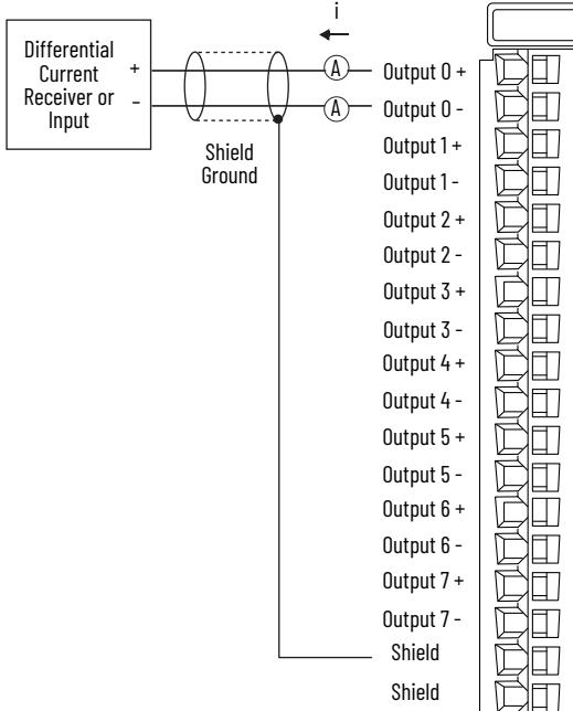
**Channel Connections** The diagram shows a device that is connected to channel 0. You are not restricted to using only this channel. You can connect devices to any channel or combination of channels as needed.
