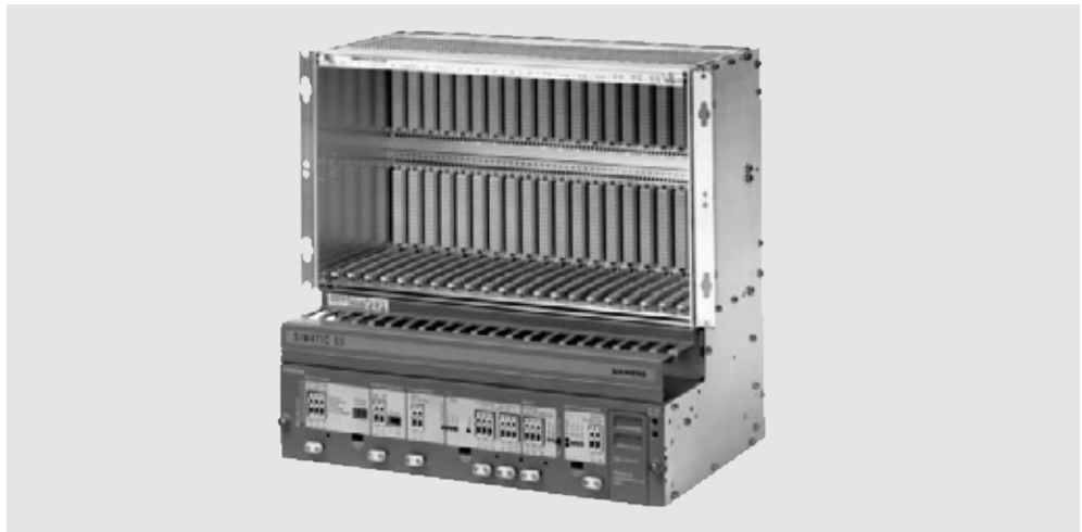
Fig. 4/1 S5-155U programmable controller
