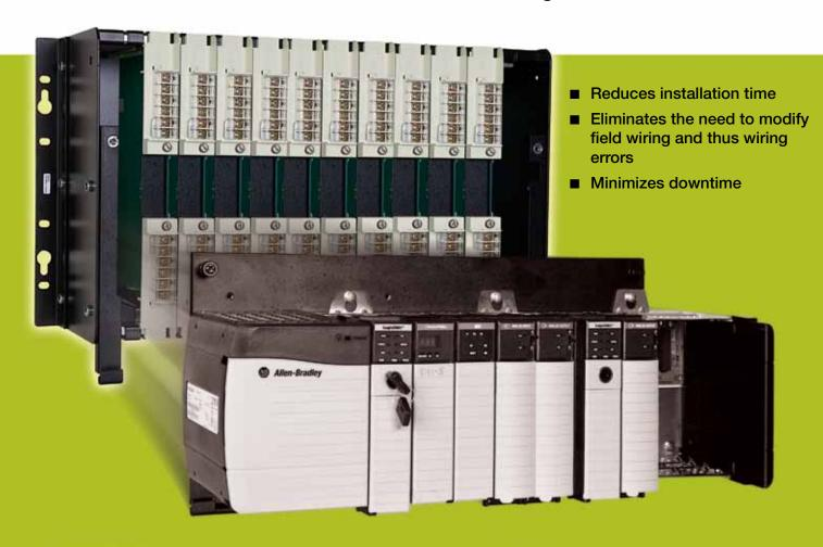
Emphatec's MIBRIDGE® offering includes an interface system to replace Honeywell's IPC-620 I/O racks. The MIBRIDGE® solution includes a chassis that replaces the IPC-620 chassis (same footprint in the control cabinet), adapter cards for 6/8, 16 and 32 channel I/O cards, and cables.
