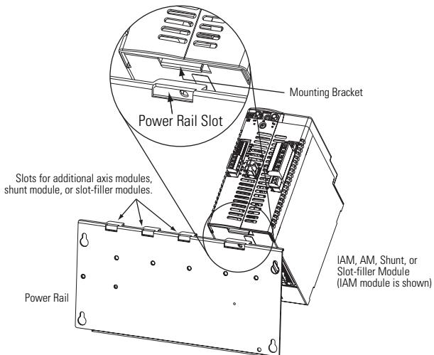
4. Pivot module downward and align the guide pins on the power rail with the guide pin holes in the back of the module.
