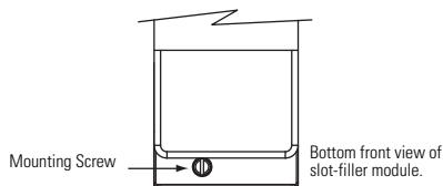
7. Repeat steps 1...6 to install a slot-filler module in each empty slot on the power rail.
