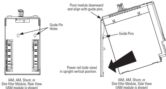
5. Gently push the module against the power rail connectors and into the final mounting position.
