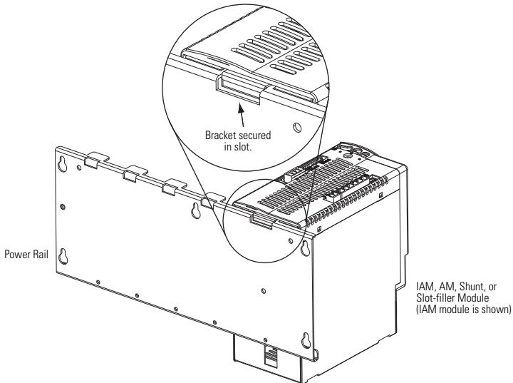
6. Use 2.26 N•m (20 lb•in) torque to tighten the mounting screw.
