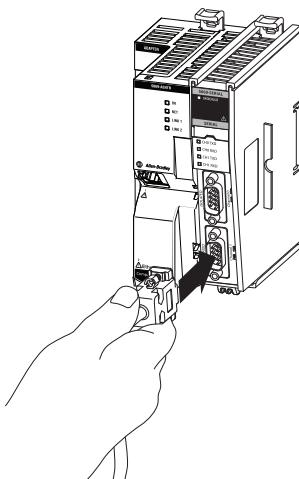
3. Tighten the screws on both sides of the serial cable.
