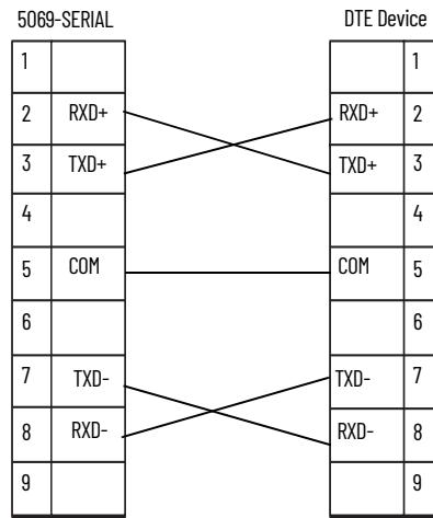
**RS-485****5069-SERIAL RS-485 Wiring**
