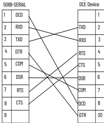
**5069-SERIAL to DTE Device with "Full or Half-duplex" or Null Modem**
