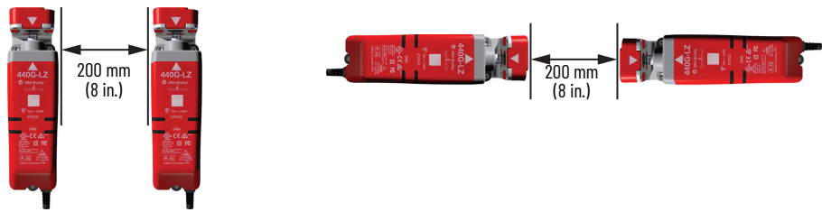
Figure 6 - Minimum Required Distance Between Two Switches
