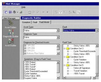
Alert Manager provides simple diagnostic configuration with easy drag and drop capabilities to quickly build fault models
