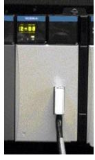
The Experion Fieldbus Interface Module (FIM) delivers robust Fieldbus device integration (Series C shown on the left, and CIOM-A FIMs shown on the right)
