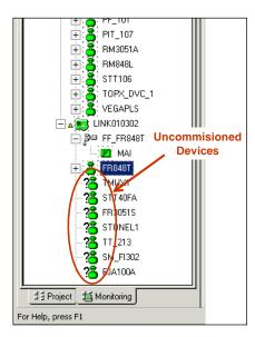
The Experion Control Builder tool provides on-line recognition of Fieldbus devices added to the link
